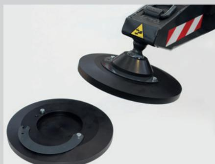
Standard pad (300 mm) with easy mounting quick coupling.
